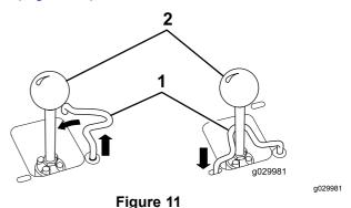
Loader arm/attachment-tilt 2. Loader-valve lock
