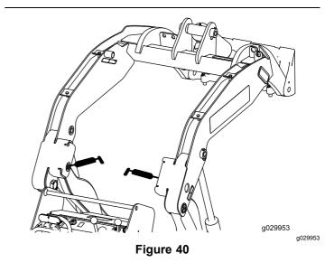
Pump grease into the fittings until grease begins to ooze out of the bearings (approximately 3
