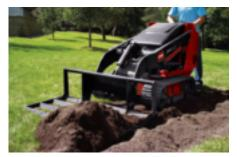
**LEVELER** Grade, finish, and spread topsoil and other landscape materials. Back fill trenches. Carry job site materials such as plants, fertilizer, irrigation supplies, and more.
