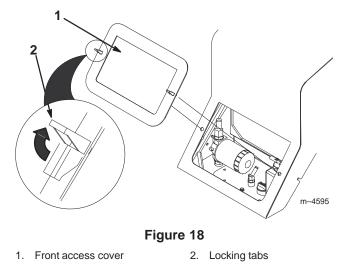
5. When finished, replace the front access cover and secure it with the two locking tabs.
