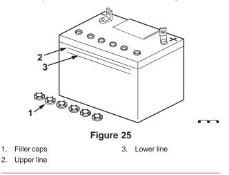
**4.** If the electrolyte is low, add the required amount of distilled water; refer to Adding Water to the Battery, page 28.
