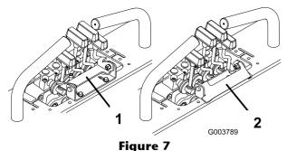
Loader valve lock, engaged
