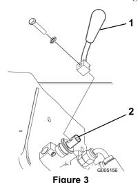
1. Speed selector valve lever 2. Speed selector valve
