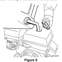
4. Add unleaded gasoline to the fuel tank, until the level is just inside the mesh filter basket.
